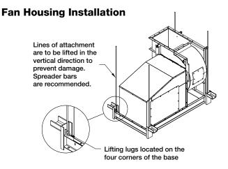
If the windband is shipped attached to the fan housing or if the windband is secured to the fan housing prior to mounting to the plenum, the fan / windband assembly should be lifted by the lifting lugs located on the fan housing. Do not lift this assembly by the lifting lugs located on the windband. Connect fan to plenum using Excelon™ flex connector found in the Vektor-CD hardware kit.
